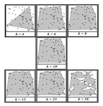
Figure 5: Output of APPROX\_k-GON() algorithm for different values of k on a randomly generated point set.
